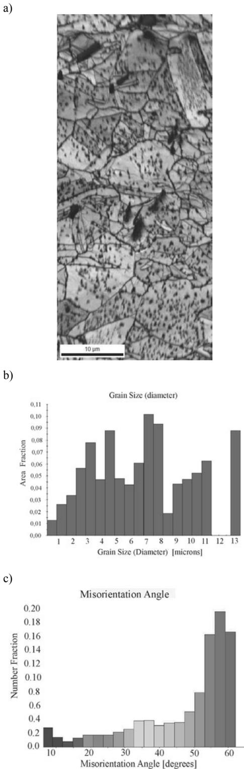
Fig. 5. Microstructure of CRCS processed (34 passes) strips of CuCr0,6 alloy (EBSD); a- IQ, b- grain size distributions, c- misorientation angle distribution
