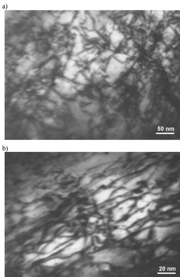
Fig. 8. Dislocation cells in CRCS processed CuCr0,6 alloy strips: a- thin foil parallel to the strip surface, b- thin foil perpendicular to the strip surface
