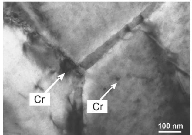
Fig. 6. Microstructure of as annealed (650 °C/1hr) CuCr<sub>0,6</sub> alloy strip –TEM
