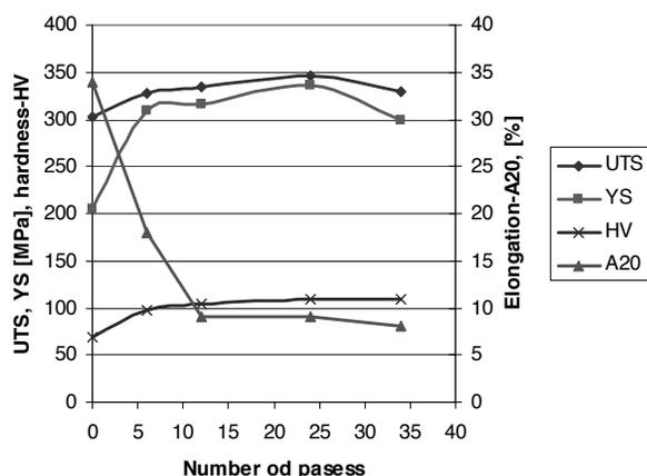
Fig. 3. Changes in mechanical properties of CuCr strips in RCS process
