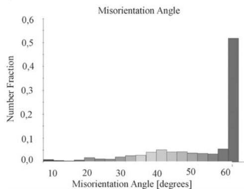
Fig. 4. Microstructure of as-annealed CuCr<sub>0,6</sub> alloy strip (EBSD): a- IQ map, b- grain size distribution, c- misorientation angle distribution
