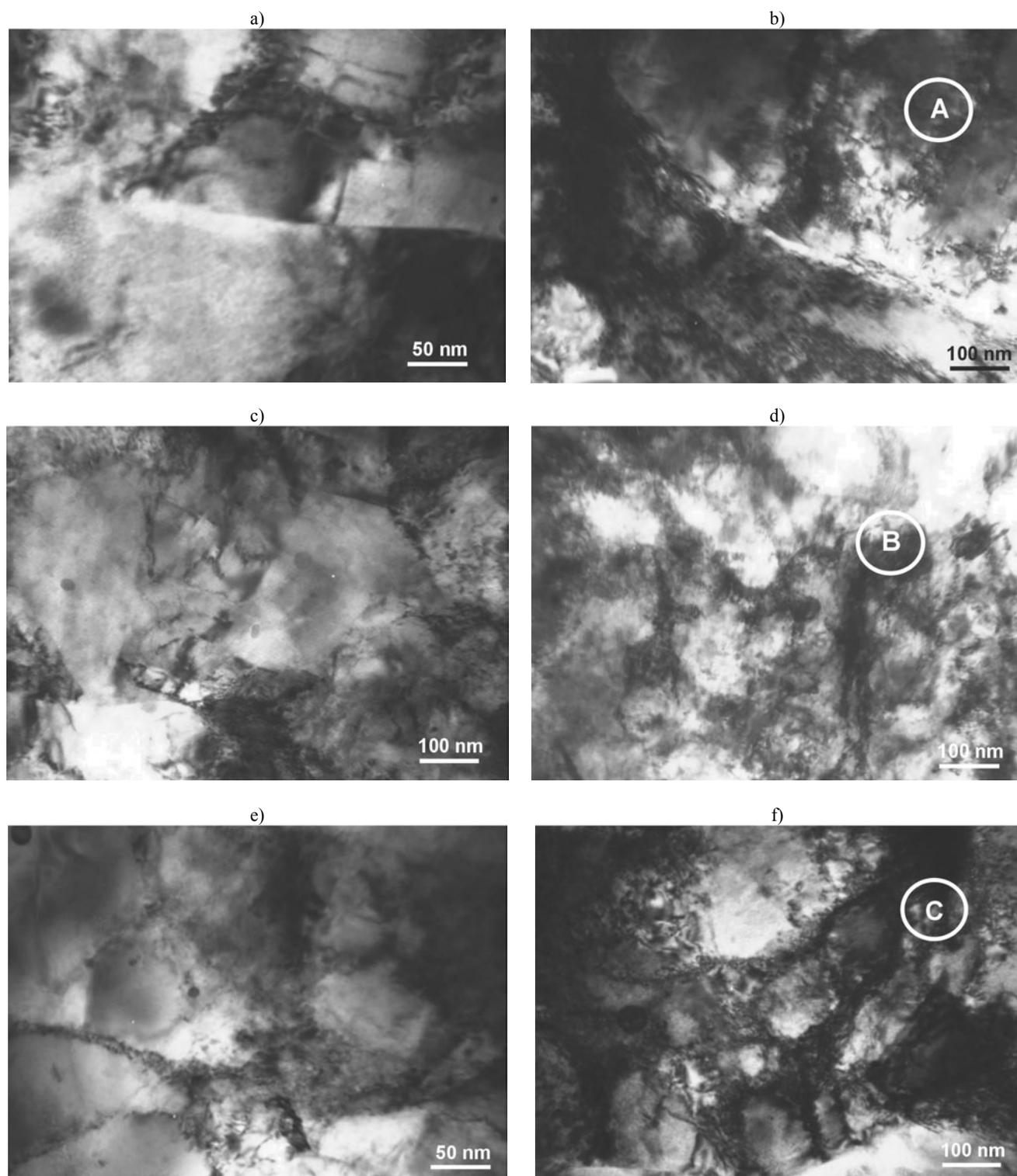
Fig. 7. TEM microstructure of CuCr<sub>0,6</sub> alloy; a, b- RCS processed (6 passes), c, d- RCS processed (12 passes), e, f- RCS processed (34 passes). Column A of RCS processed samples represents microstructures of thin foils parallel to the strip surface and column B of RCS processed samples show microstructures of thin foils perpendicular to the strip surface and along the strip
