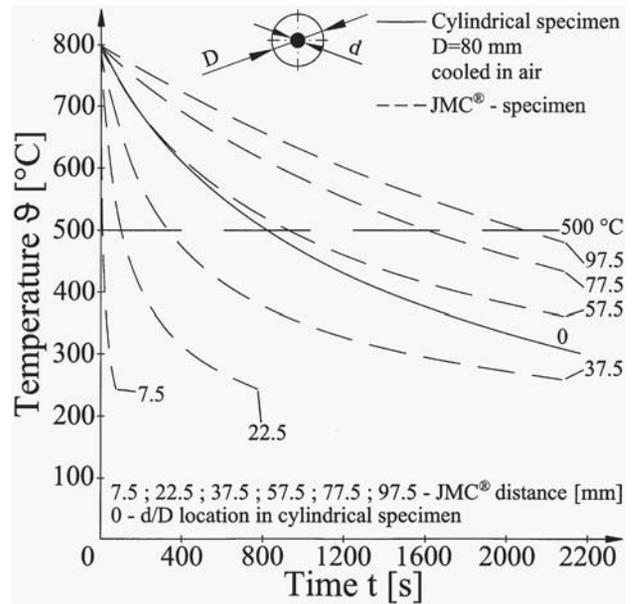
Fig. 9. Cooling curves of cylindrical specimen (D=80 mm)
