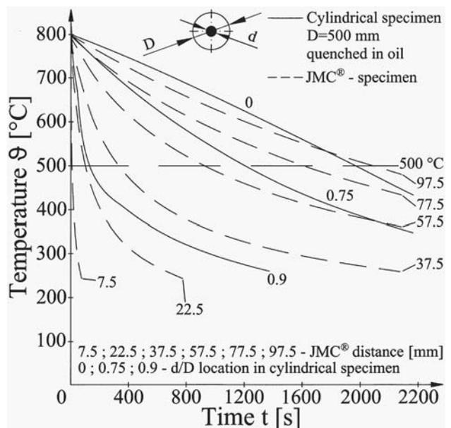
Fig. 6. Cooling curves of cylindrical specimen (D=500 mm)
