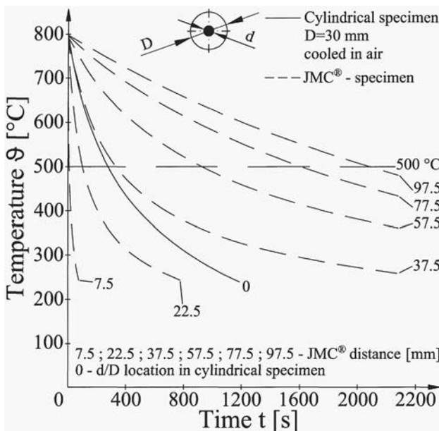
Fig. 8. Cooling curves of cylindrical specimen (D=30 mm)
