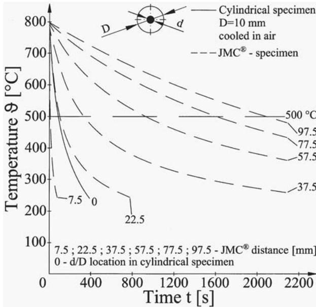
Fig. 7. Cooling curves of cylindrical specimen (D=10 mm)
