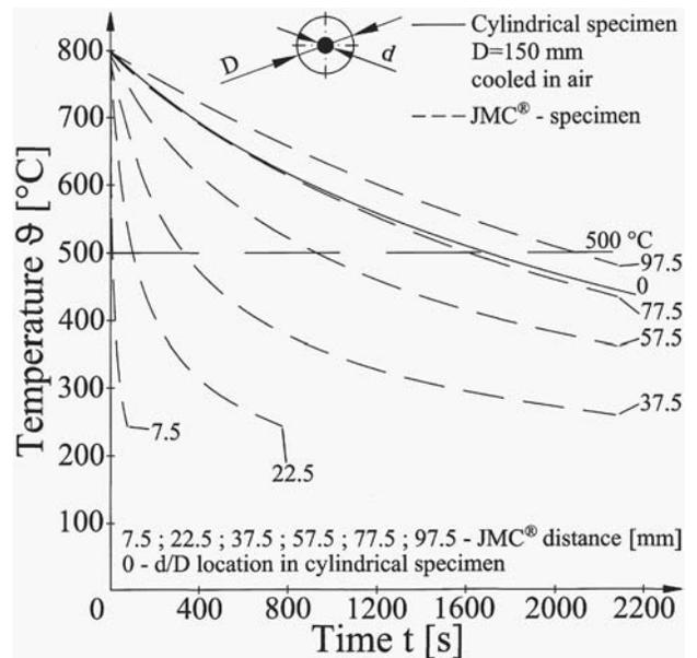
Fig. 10. Cooling curves of cylindrical specimen (D=150 mm)
