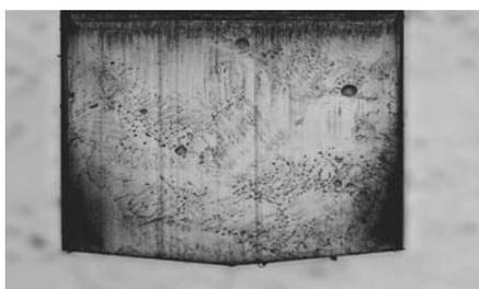
Fig. 3. The wear condition of the punch
