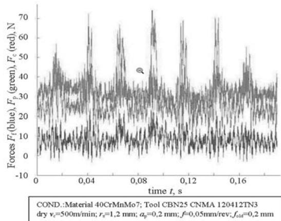
Fig. 7. Cutting forces data
