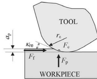
Fig. 1. Schematic presentation of tool/workpiece contact geometry
