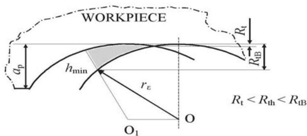
Fig. 3. Surface roughness in accordance with Brammertz (1961) [7]
