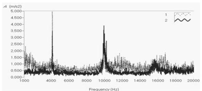
Fig. 9. The influence of tool nose radius on acceleration data,  $v_c = 450$  m/min,  $a_p = 0.2$  mm,  $f = 0.2$  mm/rev (1-  $r_n = 0.4$  mm, 2-  $r_n = 1.2$  mm)
