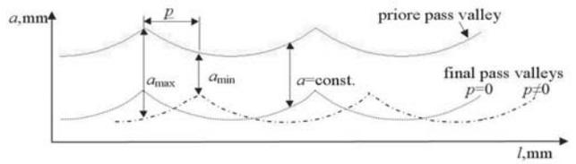
Fig. 5. Parameters for interface modeling and DOC computing
