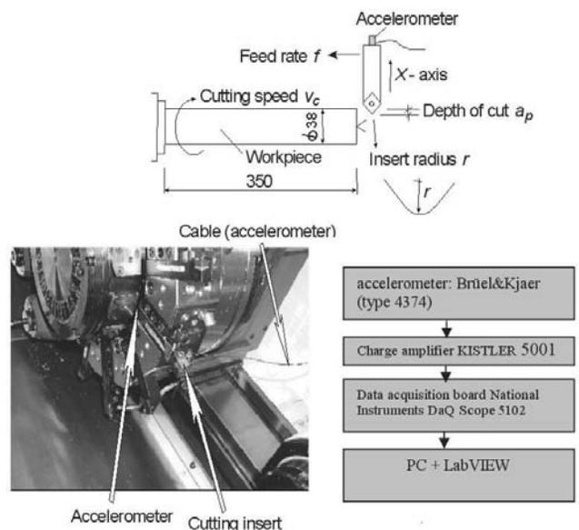
Fig. 8. Testing of significance of nose radius on dynamic characteristics of hard turning
