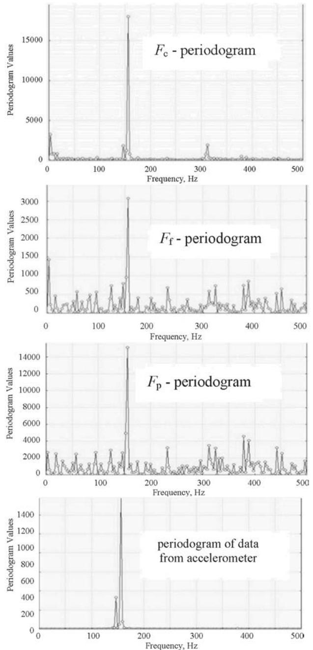
Fig. 4. Signals from accelerometers and force meters after FFT
