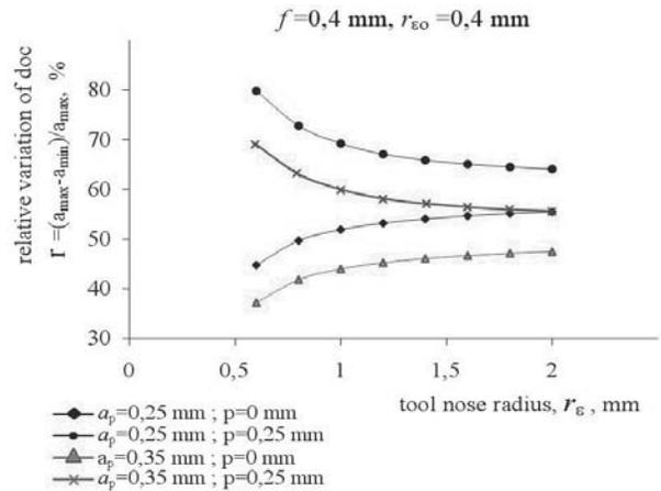
Fig. 6. Variation of DOC during hard turning
