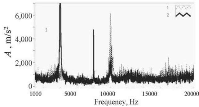
Fig. 10. The influence of cutting speed on acceleration data,  $r_e = 0.4$  mm,  $a_p = 0.2$  mm,  $f = 0.1$  mm/rev (1-  $v_c = 450$  m/min, 2-  $v_c = 550$  m/min)
