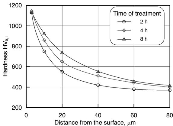
Fig. 6. Hardness profiles for the Ti-6Al-4V alloy oxynitrided at the temperature of 1173 K [35]
