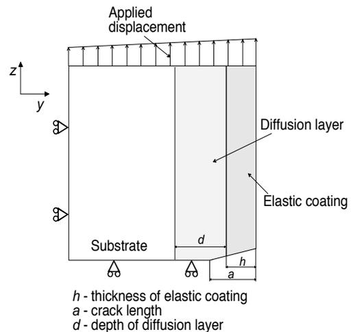
Fig. 3. Loading and boundary conditions of the FE model of the analyzed specimen segment
