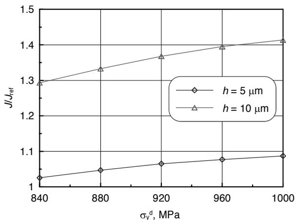
Fig. 12. The influence of the yield strength in thin diffusion layer,  $\sigma_y^d$ , on crack driving force for various coating thickness,  $h$
