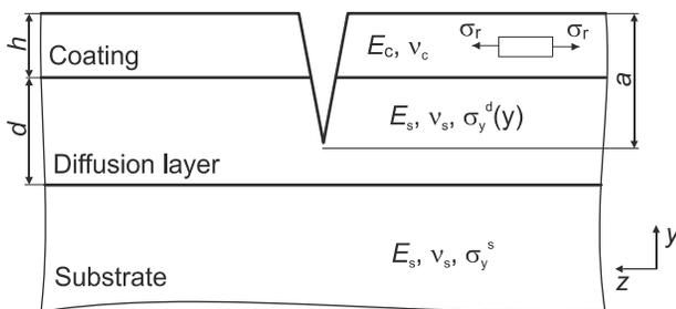
Fig. 2. The model of surface treated titanium alloy adopted for FE calculations
