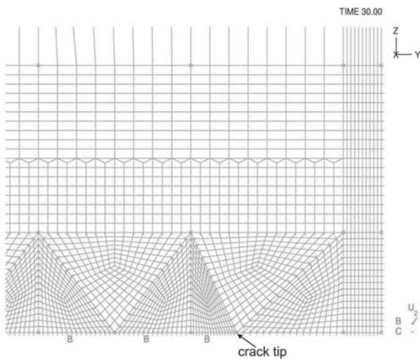
Fig. 4. FE mesh refinement in the vicinity of the crack tip
