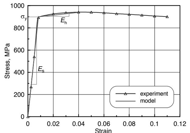
Fig. 5. Experimental stress-strain curve obtained for Ti-6Al-4V alloy and bilinear elastic-plastic relationship used in FE calculations ( $E_s$  – Young's modulus,  $E_h$  – hardening modulus)
