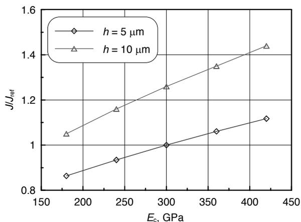
Fig. 9. The effect of coating Young's modulus,  $E_c$ , on crack driving force for various coating thickness,  $h$
