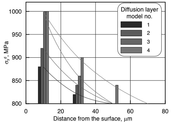
Fig. 7. Yield strength values assigned to individual sublayers in the diffusion layer; the curves represent corresponding yield strength profiles that are approximated in the models
