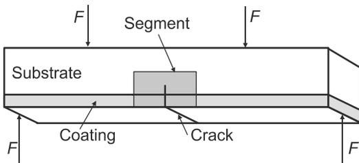
Fig. 1. Schematic diagram illustrating the four-point bending specimen with numerically analysed segment
