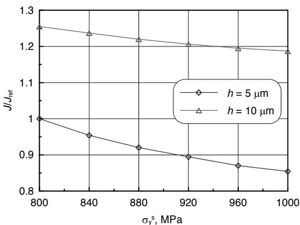
Fig. 10. The effect of substrate yield strength on crack driving force for various coating thickness
