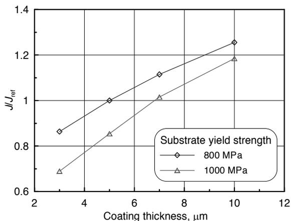
Fig. 8. The effect of coating thickness,  $h$ , on crack driving force for various yield strength of the substrate
