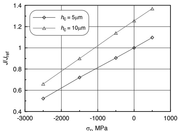
Fig. 11. The effect of coating residual stresses on crack driving force for various coating thickness
