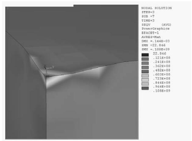
Fig. 5. Distribution of stresses after loading
