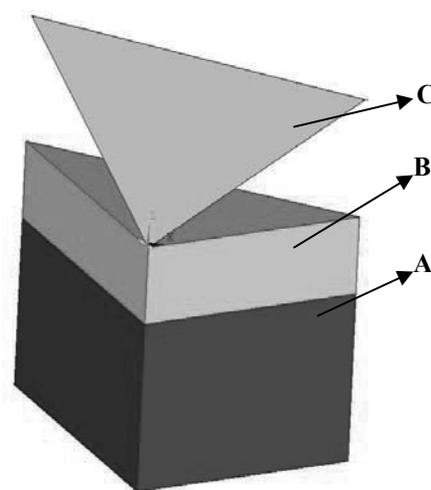
Fig. 1. Model of the sample: A - Substrate (ASP 30), B - Coating (TiN, TiC), C - Indenter Model Surface
