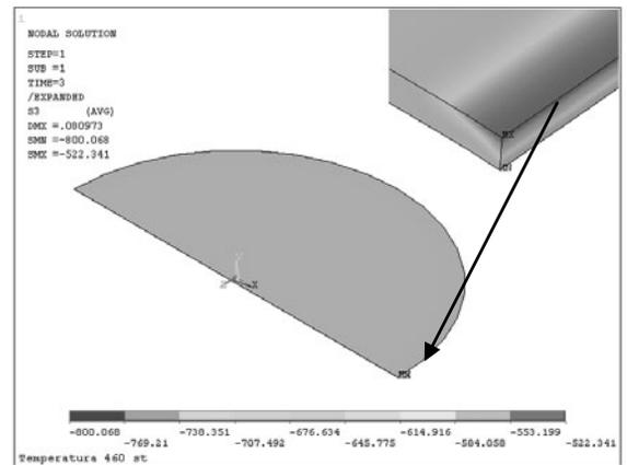
Fig. 7. Distribution of the simulated compression stresses in the TiN coating (coating thickness  $g=3.9 \mu\text{m}$ , process temperature  $460^\circ\text{C}$ , specimen distance from the magnetron disk 125 mm)
