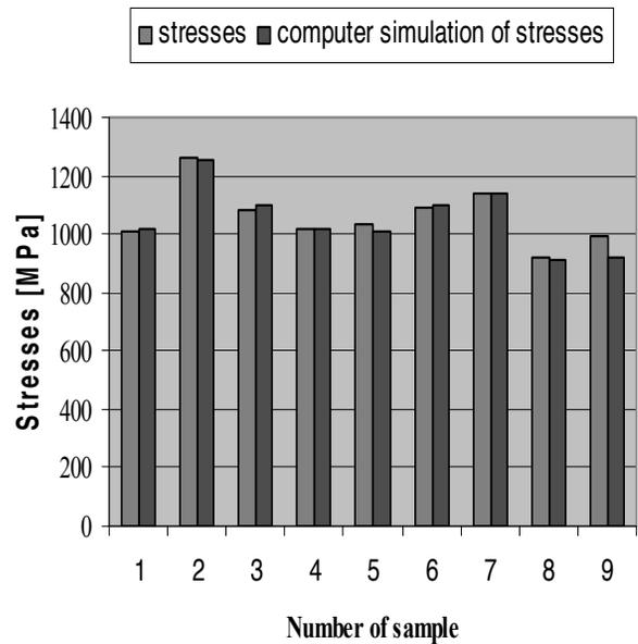
Fig. 13. Comparison of computer simulation with results of experimental investigations for stresses of TiC coatings
