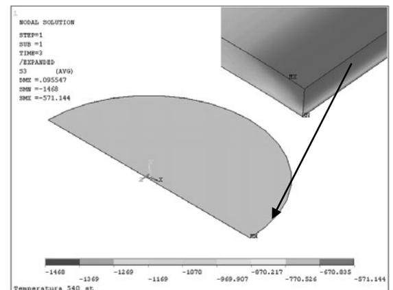
Fig. 9. Distribution of the simulated compression stresses in the TiC coating (coating thickness  $g=2.6 \mu\text{m}$ , process temperature  $500^\circ\text{C}$ , specimen distance from the magnetron disk 125 mm)
