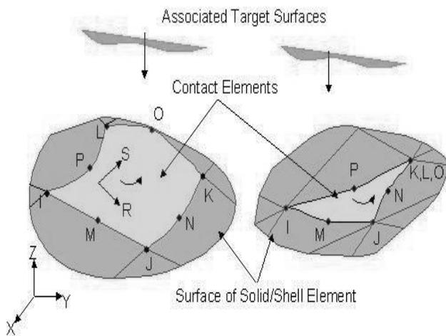
Fig. 3. Geometry and position of CONTA174 elements
