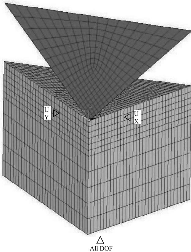
Fig. 2. Analyzed model with the overlaid finite elements mesh
