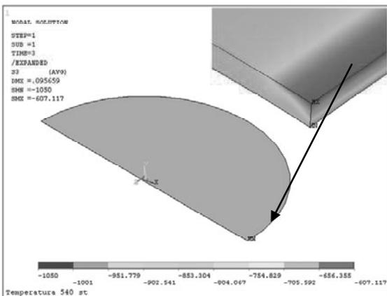
Fig. 6. Distribution of the simulated compression stresses in the TiN coating (coating thickness  $g=4.6 \mu\text{m}$ , process temperature  $540^\circ\text{C}$ , specimen distance from the magnetron disk 95 mm)
