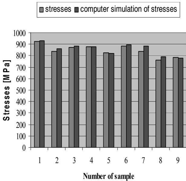
Fig. 12. Comparison of computer simulation with results of experimental investigations for stresses of TiN coatings
