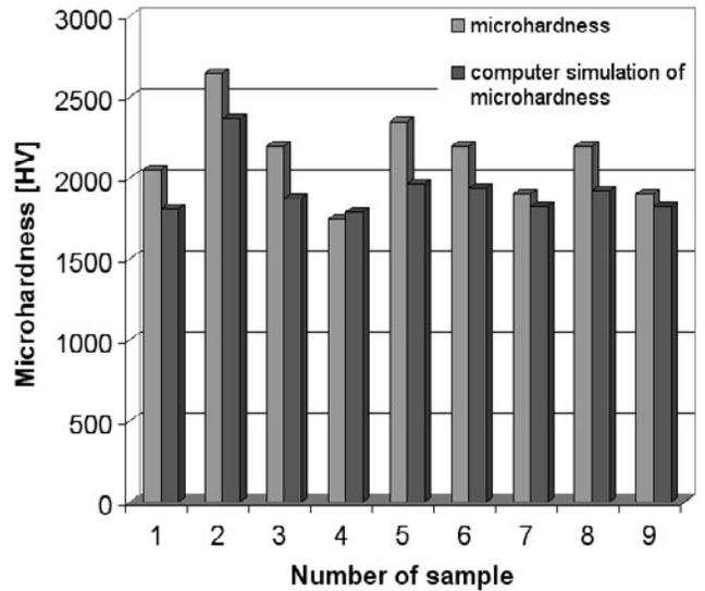
Fig. 11. Comparison of computer simulation with results of experimental investigations for microhardness of TiC coatings
