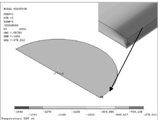
Fig. 8. Distribution of the simulated compression stresses in the TiC coating (coating thickness  $g=2.6 \mu\text{m}$ , process temperature  $540^\circ\text{C}$ , specimen distance from the magnetron disk 95 mm)
