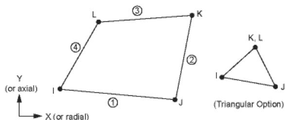
Fig. 2. Geometrical model of element FLUID141
