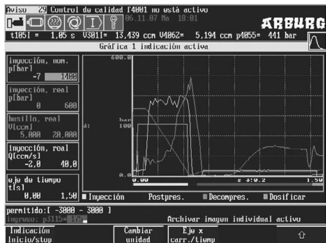
Fig. 1. Arburg injection moulding machine control panel display presenting the injection forming conditions
