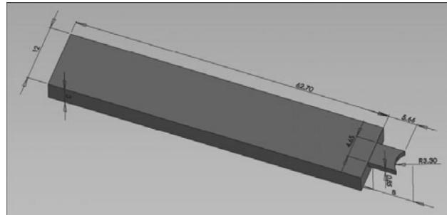
Fig. 3. Drawing of the formed green with constriction
