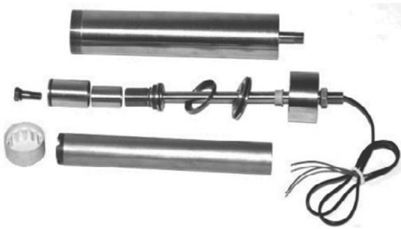
Fig. 2. Prototype MR Damper
