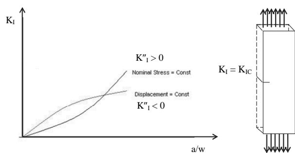
Fig. 5. Comparison of  $K_I$  value in dynamic and conventional conditions;  $K_I$  vs crack size
