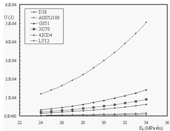
Fig. 8. Evolution of plastic strain energy,  $U$  as a function of stress intensity factor,  $K_I$
