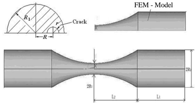
Fig. 3a. Specimen design and FEM considering of nomenclature to explain the size and geometrical position of the crack
