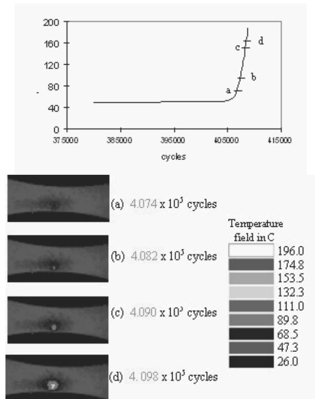
Fig. 1. Temperature field just before rupture; 42CD4 steel with stress amplitude of 460 MPa [8, 5]
