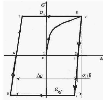
Fig. 6. Stress–strain loops under monocycle for constant strain cycling
