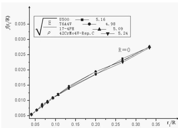
Fig. 4. Correction factor of K defined as a function of crack size for different metals
