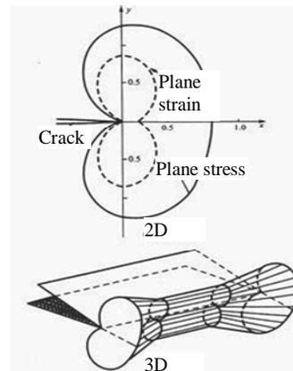
Fig. 7. 2D and 3D illustration of the crack and the plastic zone
