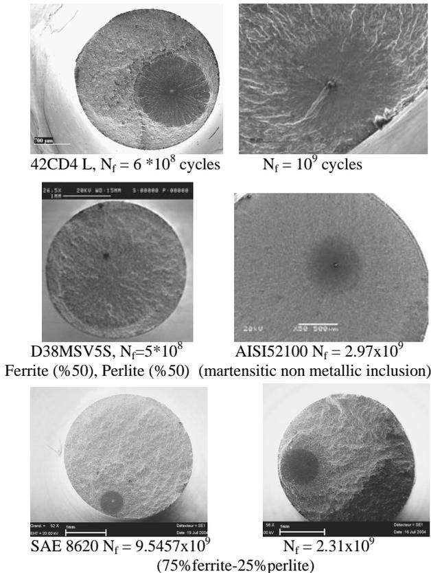
Fig. 2. Fracture surfaces of gigacycle fatigue specimens with fish eyes [6]
