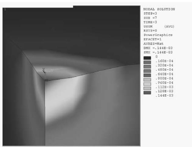
Fig. 4. State of deformed material after loading
