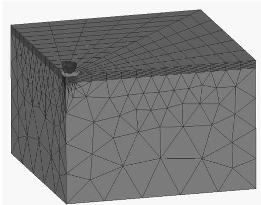
Fig. 1. Three-dimensional view of calculated model together with steel globule and put finite element mesh
